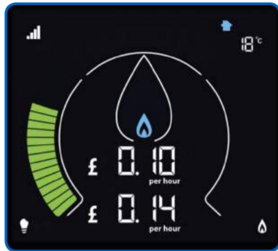
Your current usage is displayed on the left hand side of the Home screen. The outer gauge shows your electricity, and the inner flame your gas. Gas usage may take a bit longer to update – up to 30 minutes. You can use the touch-sensitive unit selectors to view your usage in pounds and pence, kilowatt hours (kWh), or carbon emissions.
